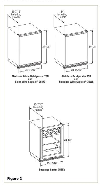
Please note that the unit has adjustable feet that can add one additional inch to height during leveling or to match adjacent cabinets (see **Figure 20** on **Page 11**).
